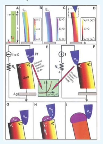
Fig. 2. Methodology to measure piezoelectric intensity by AFM. (A) Schematic definition of a NW and the coordination system. (B) Longitudinal strain distribution in the NW. (C) The corresponding longitudinal piezoelectrically induced electric field distribution in the NW. (D) Effects of the piezoelectricity on the potential field. (E and F) Contacts between the AFM tip and the sample at two reversed local contact potentials [5].
